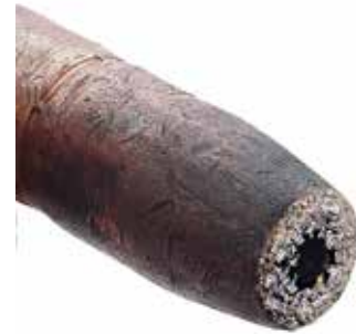
Nozzle fully clogged (not using E-WELD Nozzle)
