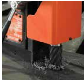
For larger holes, 1/2" and above, use the magnetic base with the standard Weldon shank
