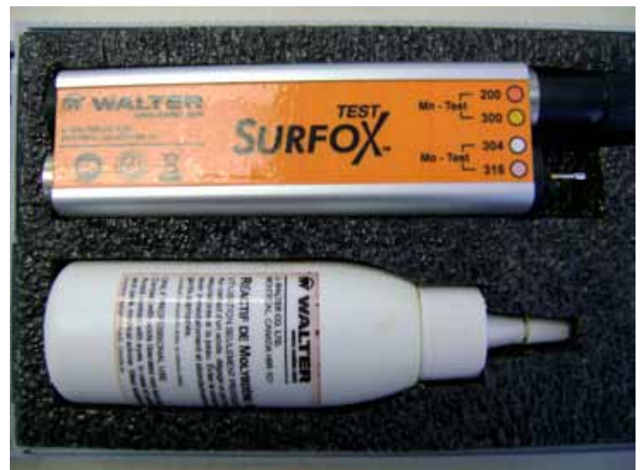
Probe and Molybdenum reagent. The Manganese reagent is inside the probe. Current is passed through the chemical solution which reacts with the surface colouring the test papers depending on the composition of the alloy.
