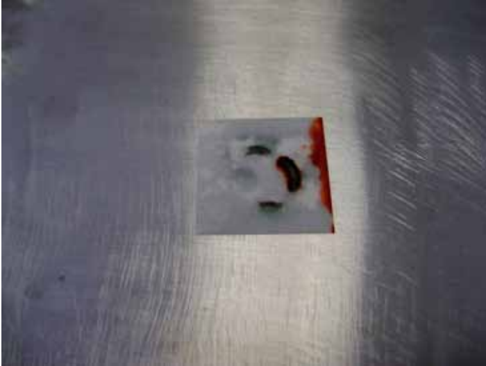
Red coloration of the test paper after probing indicates that the sample is 316 grade stainless steel. Surface has to be cleaned after the test as a deposit may be left behind.
