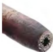
Nozzle fully clogged (not using E-WELD Nozzle)
