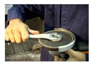
9. Always mount the Spin-On wheel using a back flange.
