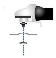
8. Tighten the wheel and make sure all is correctly in place. Do not over tighten.
