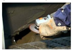
14. Always use personal protective equipment such as goggles, face shield, mask, gloves, protective clothing, etc. to prevent burns that can be caused by sparks.
