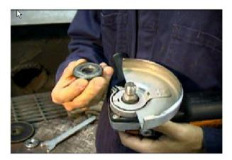
5. Make sure the back flange is well in place on the grinder's spindle shoulder.
