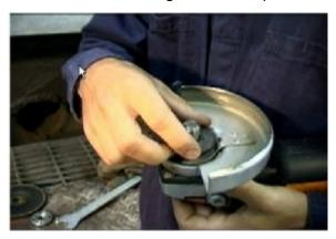
6. Make sure the wheel is placed flat on the back flange.
