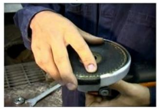
7. Center the rear nut, the grinding wheel and the tightening nut. The shoulder of the clamping nut should be oriented towards the inside of the wheel for better centering (for ¼ inch wheels).
